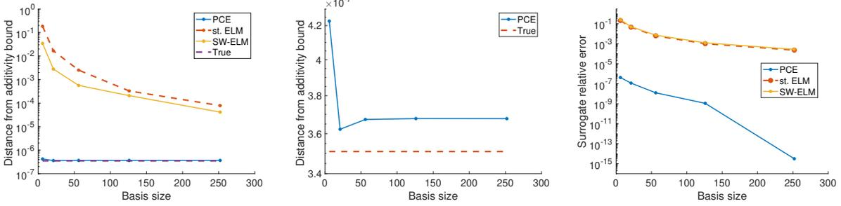
Figure 1: Low interaction case ( $10^{-6}$ ) where  $\Delta_{\text{add}} = 3.5091 \times 10^{-7}$ . **Left:** Distance from additivity bounds estimated with PCE, standard ELM, and SW-ELM. **Middle:** Distance from additivity bound for PCE only compared to true distance from additivity. **Right:** Relative error of surrogates.
