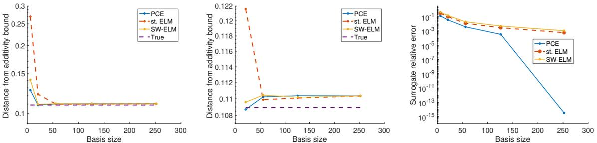
Figure 3: High interaction case ( $\delta = 10^4$ ) where  $\Delta_{\text{add}} = 0.1089$ . **Left:** Distance from additivity bounds estimated with PCE, standard ELM, and SW-ELM. **Middle:** Same as Left figure, but zoomed in. **Right:** Relative error of surrogates.
